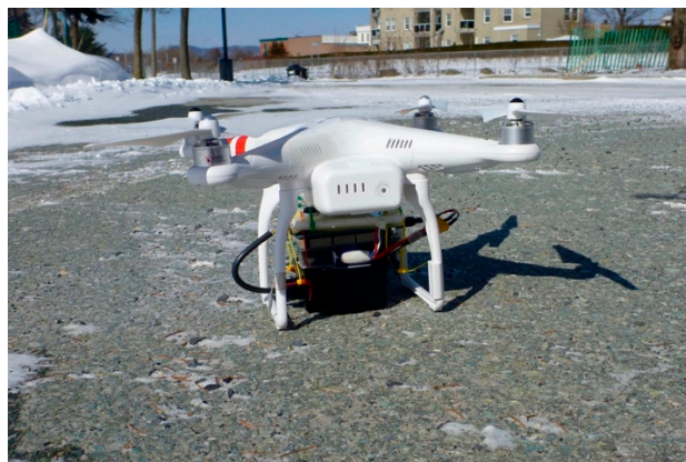
Figure 8. Radar system mounted under a Phantom 2 remotely piloted aircraft (RPA) quadcopter.
