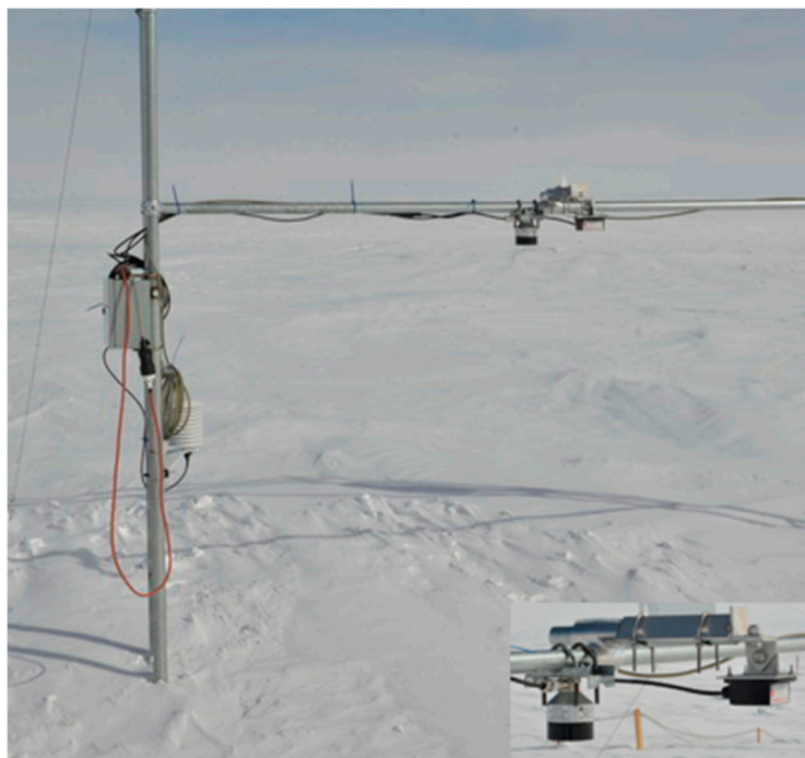
Figure 14. Set-up of the installation at Dome C, Antarctica. The horizontal mast was at 1.5 m above the snow. The close-up shows the ultrasonic snow depth sensor on the left, and the FMCW radar on the right.
