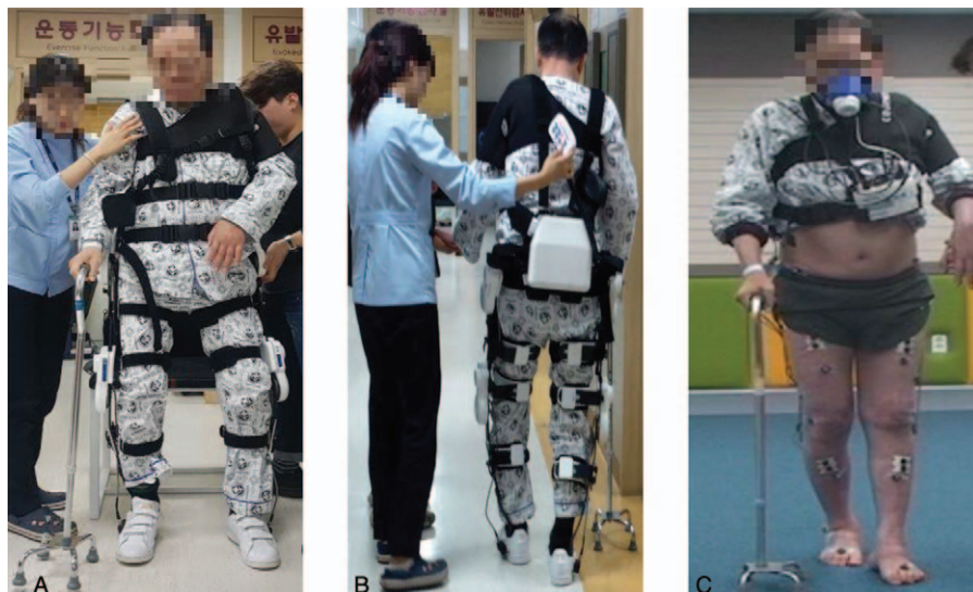
Figure 1. Robotic exoskeleton-assisted overground walking training. (A), (B) Gait training wearing Angelegs; (C) 3D gait analysis wearing portable gas analyzer.
