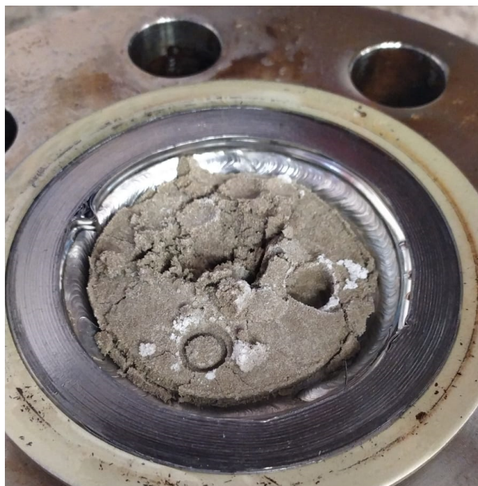
Figure 13. As soon as the test with 30.66 wt.% CuSn12 powder finished, the reactor was opened, and the medium was found to be much more compact than in the absence of powder.
