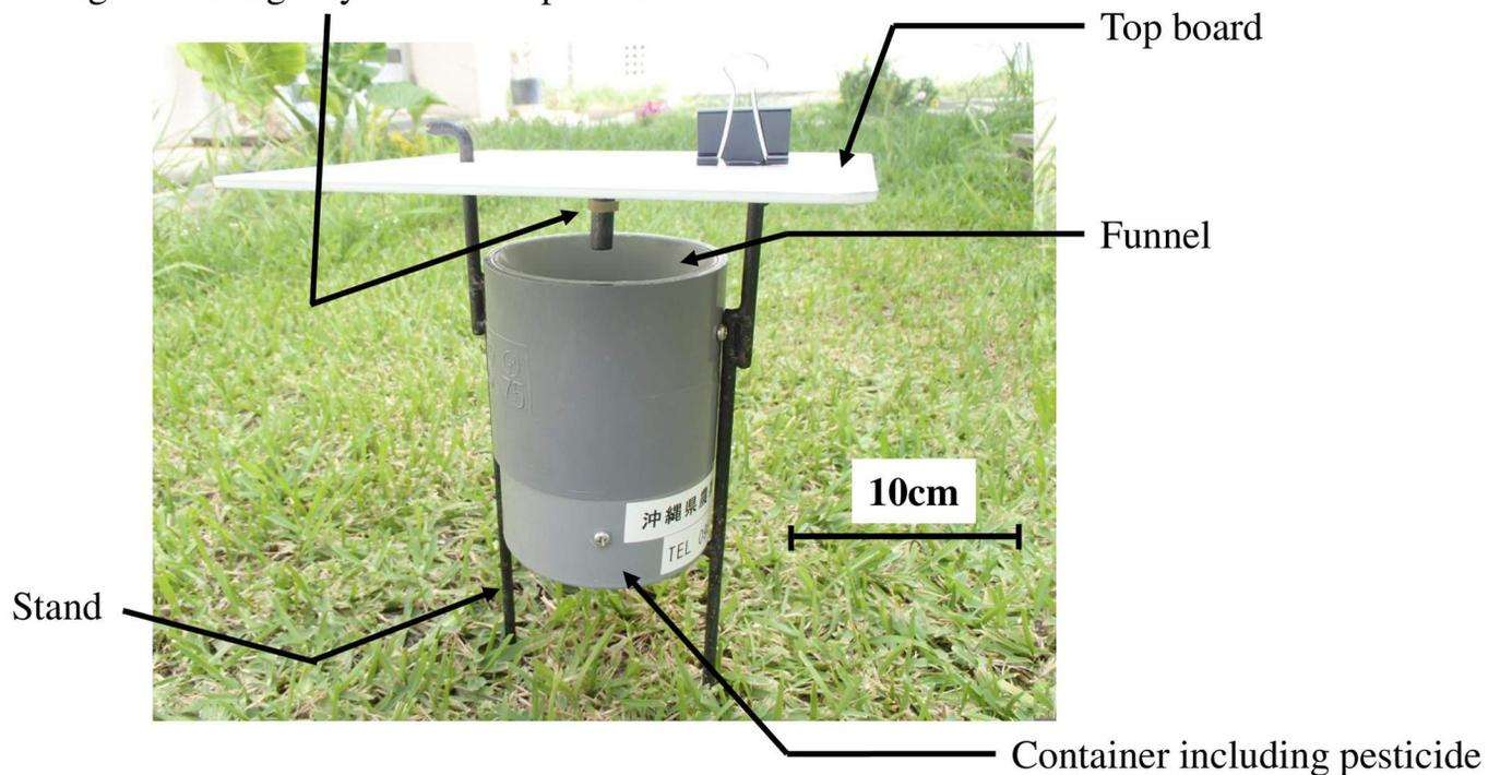
**Fig 3. Cylinder-type sex pheromone trap used after April 1998.** Traps were fitted with a rubber septum or ring containing 0.1 mg of a synthetic pheromone as an attractant. Insecticide (DDVP) was added to prevent the escape of the trapped insects.
