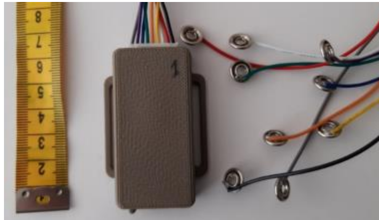
Figure 2. The data acquisition unit can measure up to eight channels and is connected to the system through snap fasteners. The unit size is 6.6 cm × 4 cm × 1.3 cm and is positioned in the front of the shoe.
