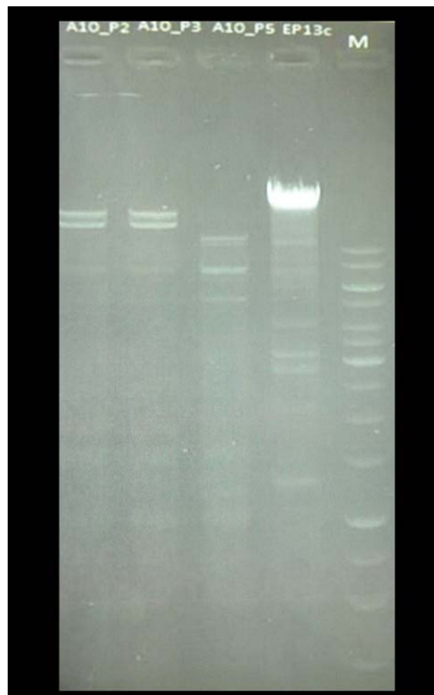
Fig. 3. Restriction with PvuII of DNA from three different E. coli phage isolates from one sampling site, drain on floor (Table 2). From left to right: slot 1, phage number 2; slot 2, phage number 3; slot 3, phage number 5; slot 4, control phage; slot 5, molecular weight marker. Phage numbers 2 and 3 gave the same restriction pattern, and phage number 5 differs from those two
