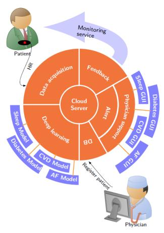
**Figure 2.** Heart Health Monitoring Service Platform (HHMSP) architecture. The common modules are in orange and the distinct modules are in blue. Abbreviations in the figure: Cardiovascular Disease (CVD), Atrial Fibrillation (AF), and Graphical User Interface (GUI).
