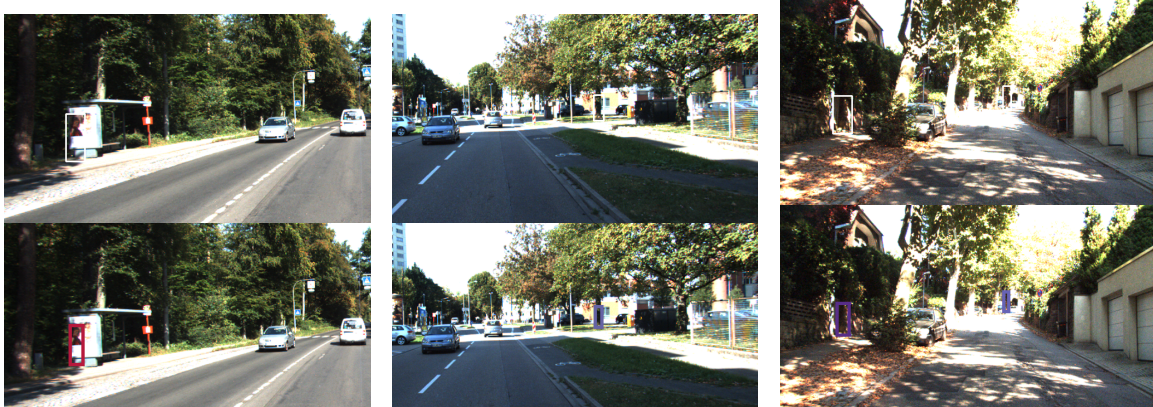
Figure 9. Examples of our tracking output in typical situations that are considered difficult in a classical tracking setup. Frames with raw pedestrian detections are shown on top of tracked pedestrians for the respective sequence. In (A), the focus is on the pair of people (green tracklets) passing with the other pair of people and coming out from a tree shadow. While their appearance changes and there is a complete occlusion, they are effectively tracked. In (B), the focus is on the person across the street who gets occluded due to the motion. Our method is able to compensate for this motion and continue tracking when he becomes visible again. In (C), we show three situations of persistent clutter where our method is tracking random objects that resemble pedestrians.
