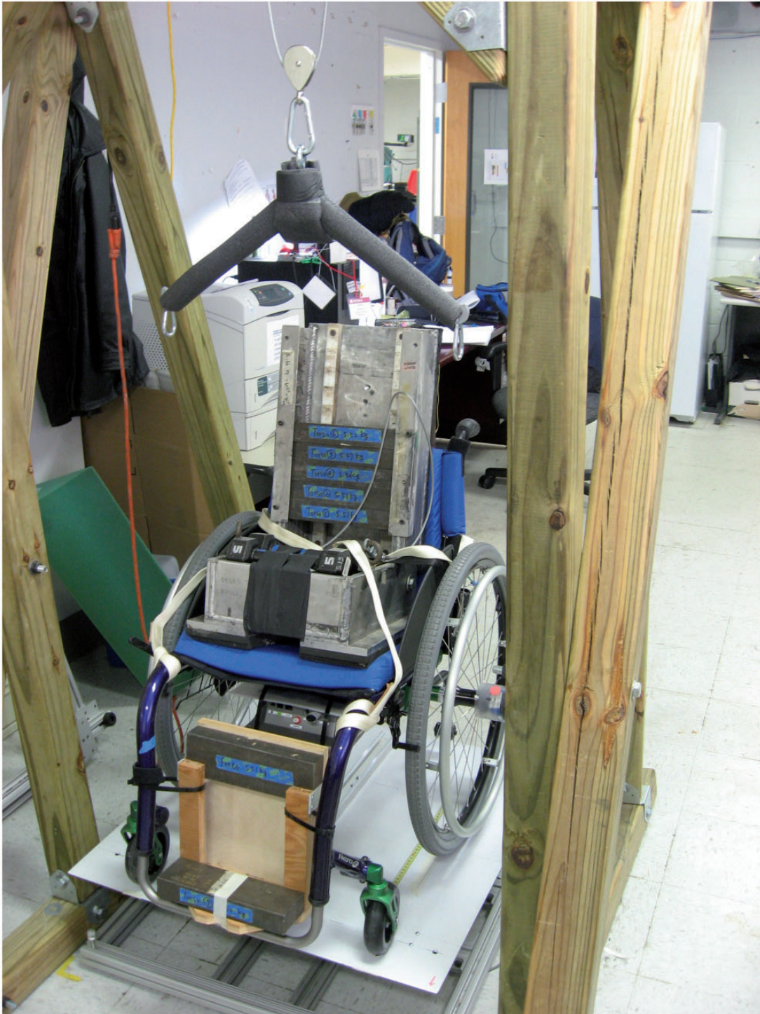
Figure 1. TiLite wheelchair loaded with ISO dummy on iMachine.
