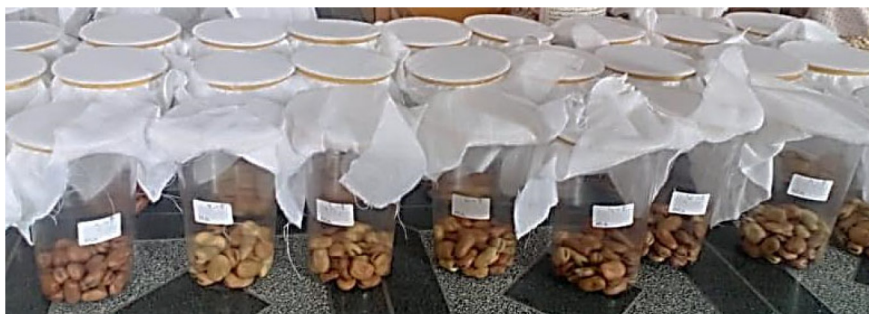
Fig. 3. Quarter- kilo plastic cups which were used in no- choice method.
