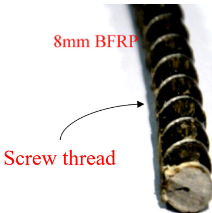
Figure 3. The BFRP bar with screw thread.
