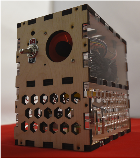
Figure 2: Building EnVironment and Occupancy (BEVO) Beacon.
