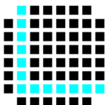
Figure 8: Representation of the "L"-shape Configuration. Squares represent individual electrodes from an MEA. Blue squares indicate electrodes used for stimulation, whereas all others are used for recording. Figure modified from reference 15 . Please click here to view a larger version of this figure.
