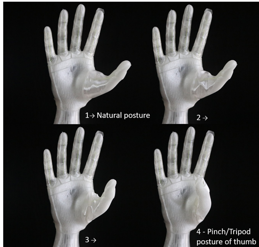
Fig 3. Articulation of thumb from natural position towards pinch/tripod position of the thumb. While moving from position 1 to 4, in coordination with other fingers, it is able to perform power grasp.
