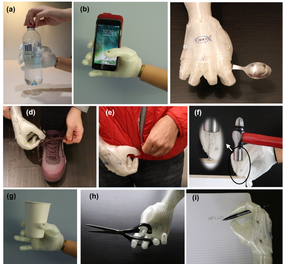
Fig 14. X-Limb performing three grasp types for carrying out AM-ULA tasks: Power grasp (a,b,c), pinch grasp (d, e,f) and tripod grasp (g,h,i).
