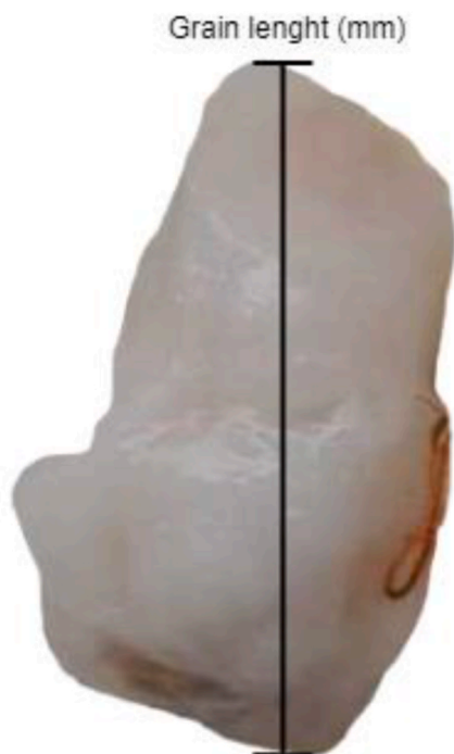
Fig. 3. Measurement of grain length using a digital king foot.
