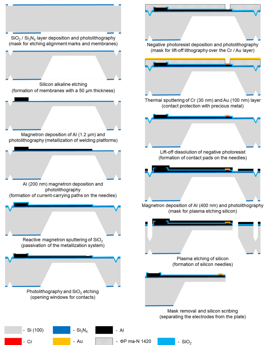
Figure 2. Technological route for the manufacture of multi-electrode array.
