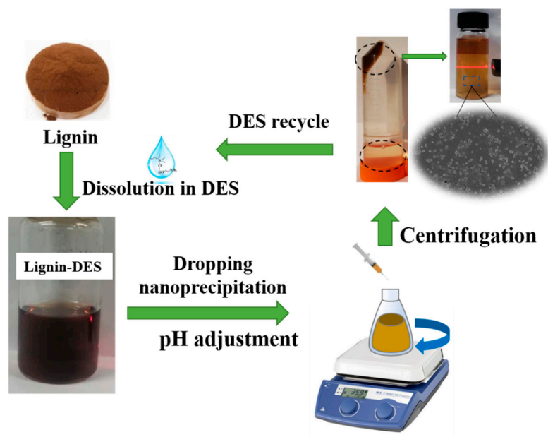
Figure 1. Schematic representation of the preparation procedure of lignin nanoparticles (LNPs). DES: deep eutectic solvent.
