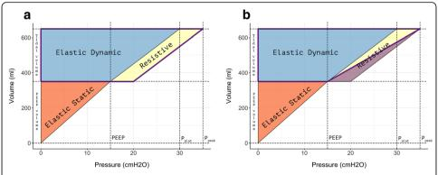
**Fig. 2** Geometrical view of mechanical power for volume-controlled ventilation. Left pane (a) I: the violet contoured trapezoid represents the mechanical power as calculated with the reference formula (Eq. 1). Right panel (b): the violet contoured trapezoid represents the mechanical power as calculated with our unadjusted surrogate (Eq. 3). The violet-filled triangle represents the bias (Eq. 4) between our unadjusted surrogate (Eq. 3) and the reference formula (Eq. 1)
