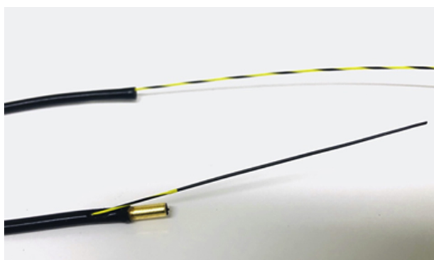
Figure 2. A custom-made gold-plated neodymium magnet, 3 mm in diameter, was loaded onto a 10F stent pusher. A side hole was created on the pusher using a surgical blade to facilitate over-the-guidewire insertion.
