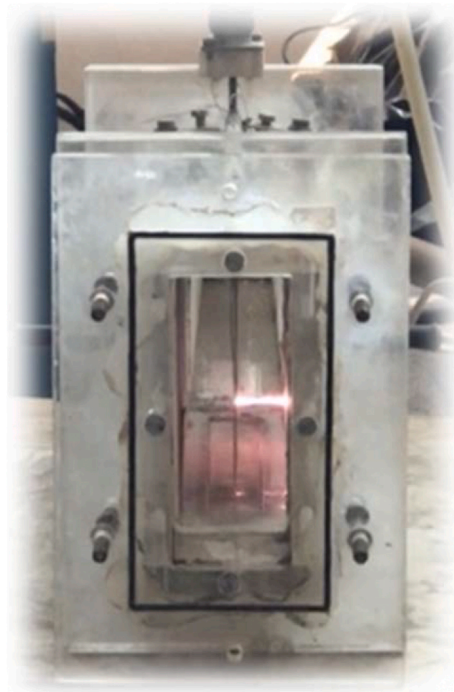
Fig. 5. The exact moment of generated electrical arcs.
