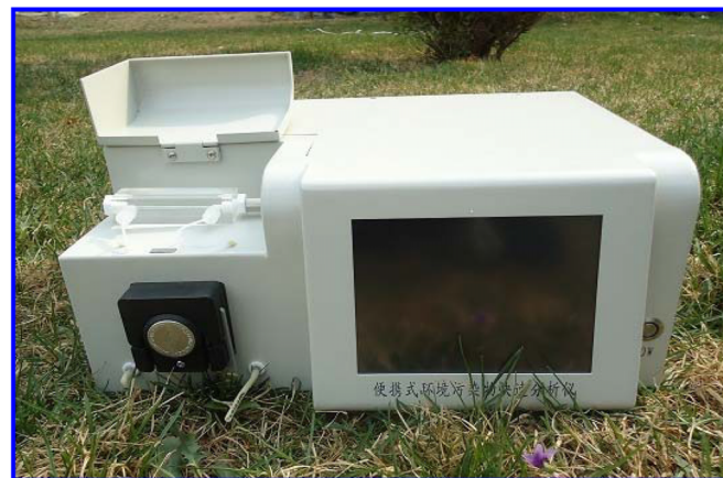
Figure 1 | (A) Schematic of evanescent wave all-fiber optical biosensing platform. (B) Photograph of the biosensing platform for the on-site/ in situ detection of heavy metal ions. (Photo by Feng Long).
