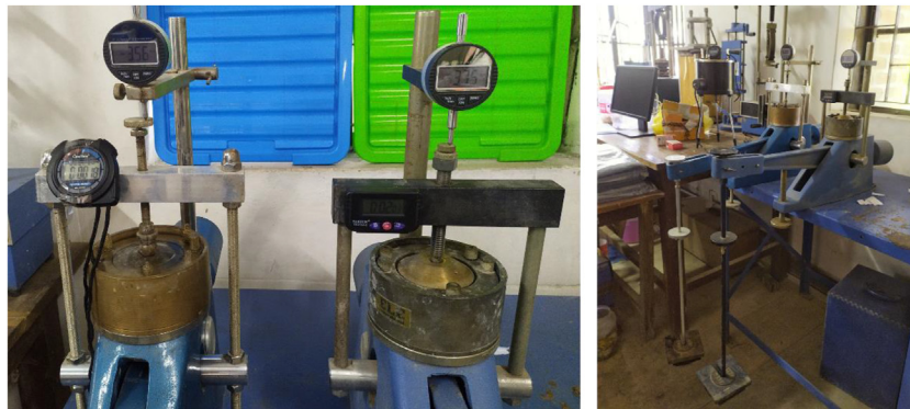
Figure 2. Consolidation test set up used in this research.
