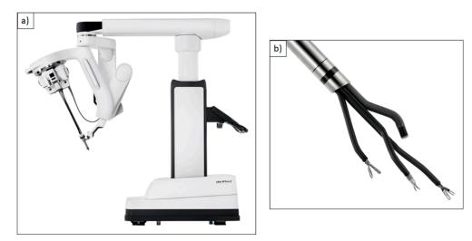
**Figure 3.** (a) DaVinci Single-Port (SP)<sup>®</sup> robotic system; (b) Single 2.5 cm cannula containing three instrument arms and an endoscope. Reproduced with kind permission from Intuitive Surgical<sup>®</sup>, Inc., Sunnyvale, CA, USA, © 2021.
