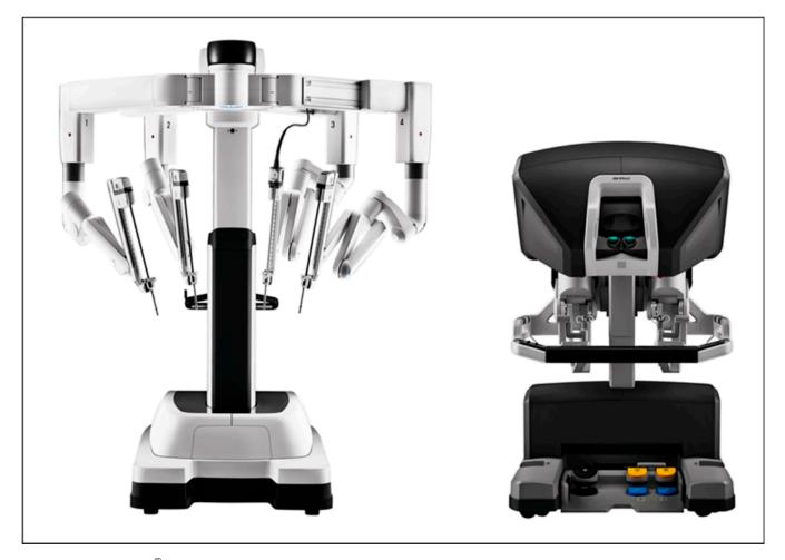
**Figure 1.** DaVinci Xi<sup>®</sup>. Multi-port robotic system with camera arm and several working arms for the use of different surgical instruments. Reproduced with kind permission from Intuitive Surgical<sup>®</sup>, Inc., Sunnyvale, CA, USA, © 2021.
