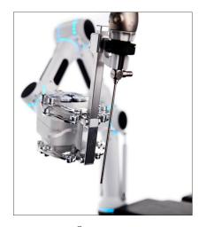
**Figure 6.** Cirq<sup>®</sup>. Robot-assisted endoscope guidance system with a mechatronic arm consisting of several segments with 7 degrees of freedom and the possibility to attach a conventional endoscope. Reproduced with kind permission from Medineering/Brainlab<sup>®</sup>, Munich, Germany, © 2021.
