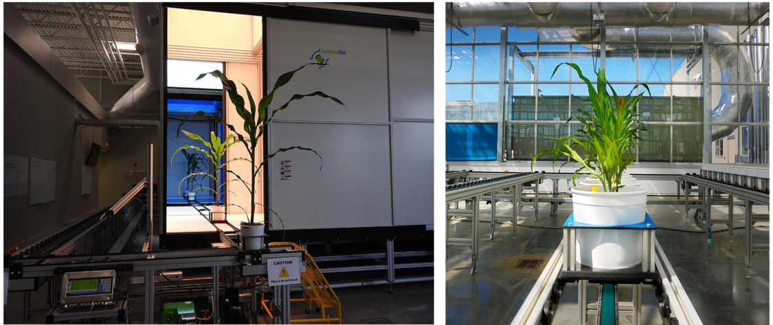
Fig 1. The proposed dataset, CosegPP , was collected using the LemnaTec Scanalyzer 3D plant phenotyping facility located at the University of Nebraska-Lincoln, USA. This facility is meant to create high throughput plant phenotyping datasets. The first image shows plants being imaged with a visible, infrared, fluorescent, and near infrared camera and exiting the LemnaTec chambers. The second image shows a row of plants on a conveyor belt in the greenhouse located next to the LemnaTec chamber.
