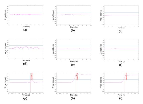
**Figure 6.** Roll angle graphs. Less-dynamic motions: (a) walking, (b) climbing up and down the stairs, and (c) slowly sitting the on stool and getting up. Highly dynamic motions: (d) jogging, (e) quickly sitting on the chair and getting up, and (f) quickly sitting on low-height mattress and getting up. Fall motions: (g) backward fall, (h) lateral fall, and (i) twist fall.
