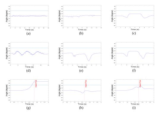
**Figure 7.** Pitch angle graphs. Less-dynamic motions: (a) walking, (b) climbing up and down the stairs, and (c) slowly sitting on the stool and getting up. Highly dynamic motions: (d) jogging, (e) quickly sitting on the chair and getting up, and (f) quickly sitting on low-height mattress and getting up. Fall motions: (g) backward fall, (h) lateral fall, and (i) twist fall.
