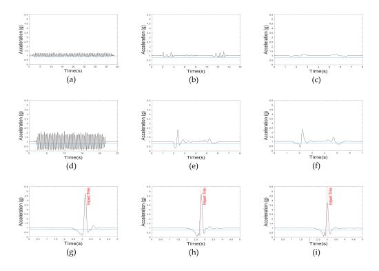
Figure 8. Acceleration SVM graphs. Less-dynamic motions: (a) walking, (b) climbing up and down the stairs, and (c) slowly sitting on the stool and getting up. Highly dynamic motions: (d) jogging, (e) quickly sitting on the chair and getting up, and (f) quickly sitting on low-height mattress and getting up. Fall motions: (g) backward fall, (h) lateral fall, and (i) twist fall.
