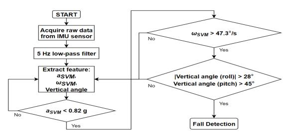
Figure 10. Flow chart of the proposed algorithm.
