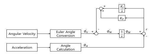
Figure 5. Gyroscope-Accelerometer fusion complementary filter with a PI controller.
