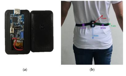
Figure 3. (a) IMU and (b) sensor position.
