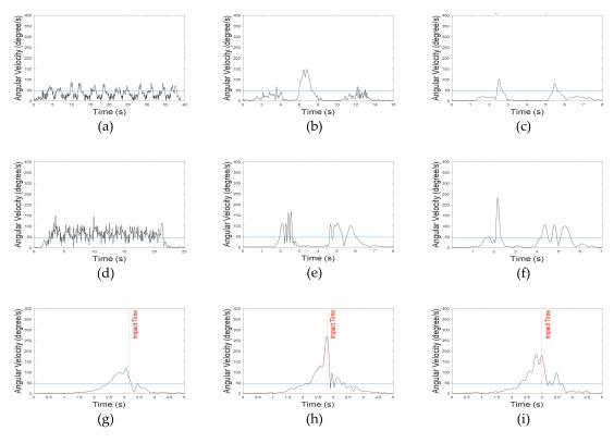
**Figure 9.** Angular velocity SVM graphs. Less-dynamic motions: (a) walking, (b) climbing up and down the stairs, and (c) slowly sitting on the stool and getting up. Highly dynamic motions: (d) jogging, (e) quickly sitting on the chair and getting up, and (f) quickly sitting on low-height mattress and getting up. Fall motions: (g) backward fall, (h) lateral fall, and (i) twist fall.
