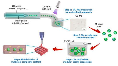
**Figure 7.** Flowcharts of microfluidic and 3D printing for the preparation of hydrogel neural scaffolds. (Reprinted with permission from Ref. [172]. 2020, Elsevier).
