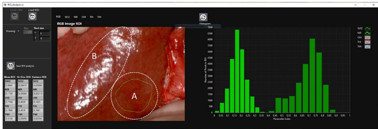
FIGURE 1. Exemplary picture of the image analysis using the TIVITA Suite Tissue software (Diaspective Vision GmbH, Am Salzhaff-Pepelow, Germany). The ROI for measurement of StO 2 , near-infrared perfusion index, organ hemoglobin index, and tissue water index was manually defined (A). Areas with light reflection artifacts were avoided (B). ROI, region of interest.
