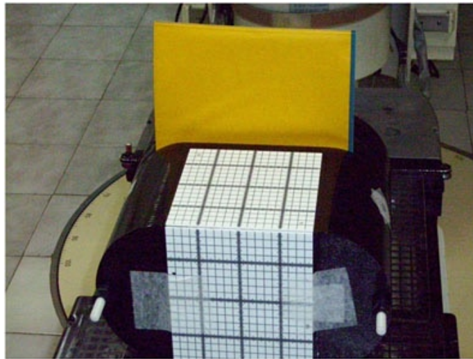
FIG. 3. Final assembly of the locally fabricated IMRT phantom.
