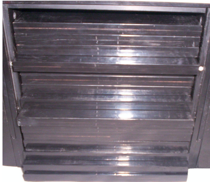
FIG. 2(c). Photograph of radiochromic film holder.
