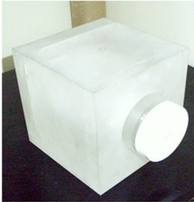
FIG. 2(a). Holder for gel dosimeter container.
