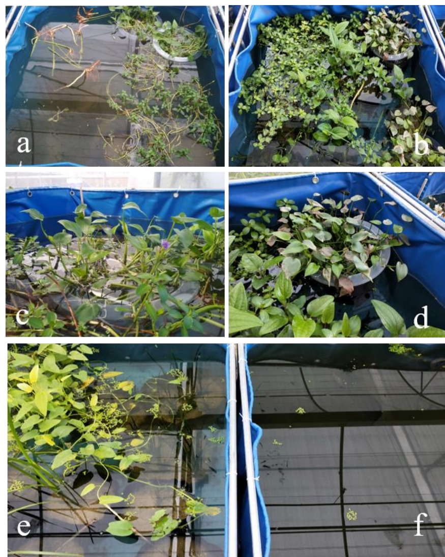
Figure 5. Growth status of plant combinations in wastewater: (a) day 0 and (b) day 27 of group A; (c) day 8 and (d) day 27 of M. vaginalis ; (e) day 35 of group B; (f) day 35 of the CK group.
