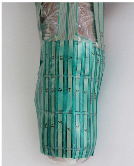
Figure 4. Four F-socket transducers covering all aspects of the residual limb to give an overall impression of pressure distribution inside transtibial prosthetic sockets [92].
