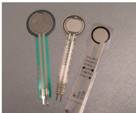
Figure 3. Three common types of FSRs: Interlink, LuSense, and FlexiForce [85].
