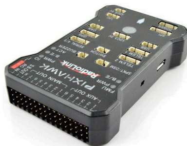
Figure 5. Pixhawk controller for fixed-wing UAV.
