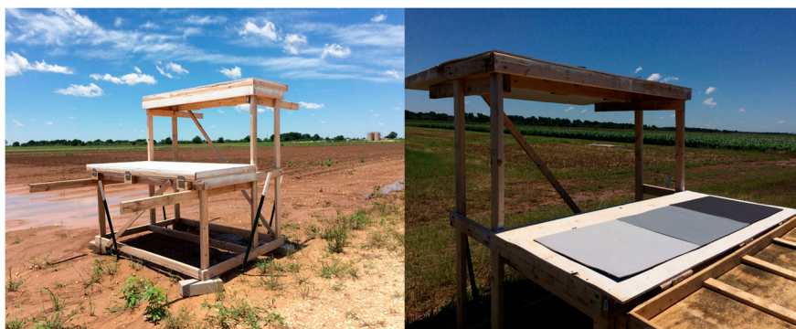
Figure 6. Ground control points set up in the field for geo-referencing, radiometric calibration, and crop height calibration (Photo Credit: Cody Bagnall).
