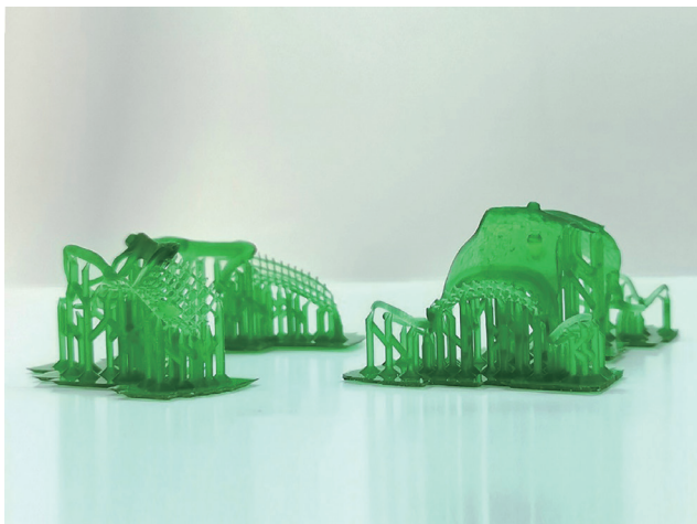
Fig. 3. Removable partial denture frameworks after 3D printing and curing from castable resin and before removal of the support structure.
