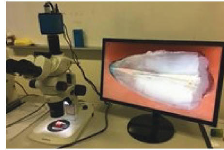
FIGURE 1: Methylene blue penetration was observed under a stereomicroscope with 8x magnification. The penetration of the methylene blue solution was observed in the apical region.
