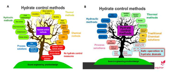
**Figure 3.** Equinor's concept of hydrate flow assurance best practices in 2014 (**A**) and 2019 (**B**). Note the lower rightmost methods, are trending toward a "do nothing" strategy (Li, et al., [26]).
