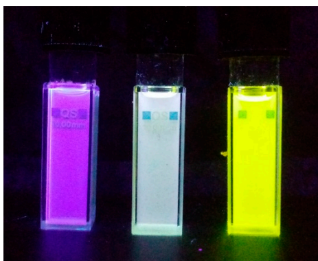
Figure 5. Changes in the color of a dichloromethane solution of 2c ( c = 1.25 \times 10^{-5} M) after the addition of 45 equivalents (middle) and in 10^{-2} M CSA (right). Photographs were taken in the dark upon irradiation with a hand-held UV lamp ( \lambda_{\text{em}} = 366 nm).
