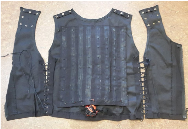
Fig. 1 The tactile vest with a 40-mm inter-tactor spacing (used in experiments 1–4)
