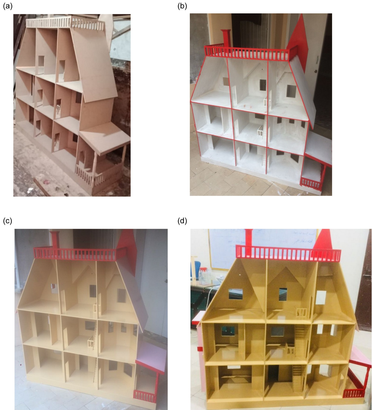
Fig 2. Pictures of the design process of the smart home prototype, (a) side view of initial design with the base color, (b) primer paint on the prototype, (c) first coating of the selected color, and (d) the prototype in its finished form with the selected color.
