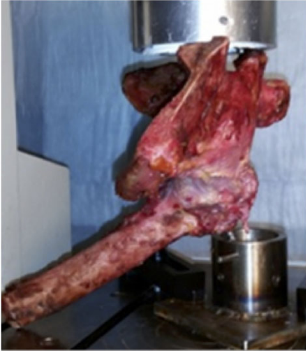
Fig. 1. Representative cadaveric hip experimental setup prior to performing capsulotomy. The femoral and pelvic sides of the specimen were secured with metal bolts and potted in poly-methyl methacrylate cement within 3-inch diameter polyvinyl chloride pipes. They were positioned in neutral hip position in a materials testing system.
