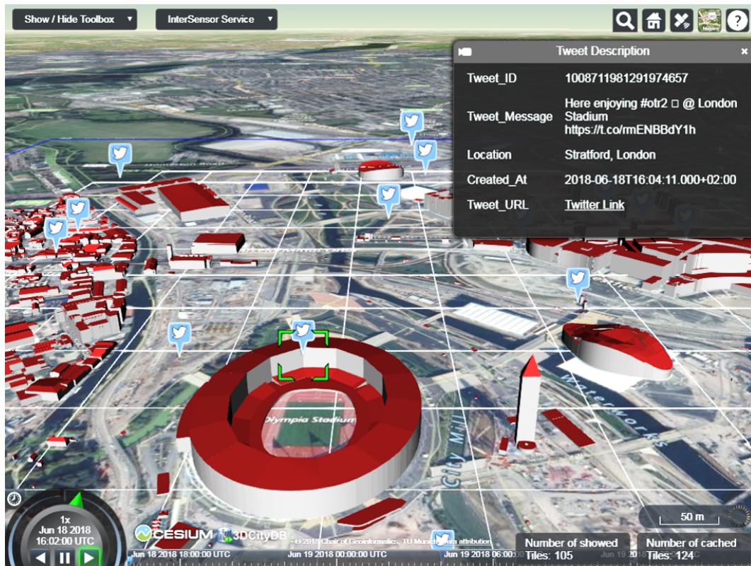
Figure 10. Joint visualization of geo-tagged tweets retrieved by the InterSensor Service along with CityGML-based 3D building objects in the district Queen Elizabeth Olympic Park, London. Screenshot taken from 3DCityDB-Web-Map application [91].
