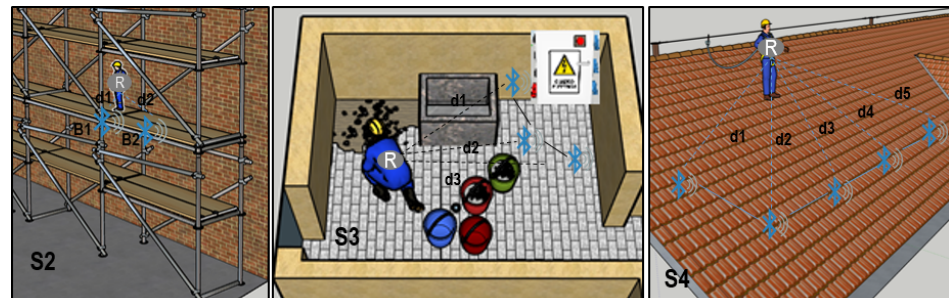
Figure 10. Different usage scenarios of the virtual fence on scaffolding task (S2), with electric risk (S3) and roofing (S4).
