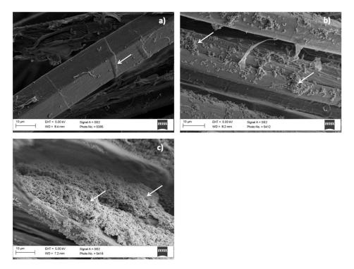
**Figure 2.** SEM pictures reporting different stages of bacterial adhesion and biofilm formation on flax fibers. Single cells of *S. aureus* adhered onto the substrate (**a**); initial steps of biofilm formation locally aggregated onto the surface of the fiber (**b**); dense structured biofilm completely covering the flax substrate (**c**).
