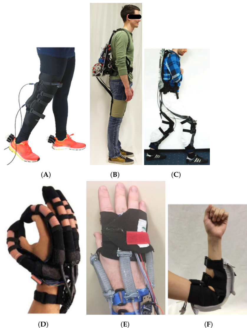
Figure 3. Wearable assistive robots with soft structure. Lower limb assistive robots: (A) soft-inflatable knee exosuit for rehabilitation [42] (Licensed under (CC BY 4.0)), (B) soft exosuit for hip assistance [44] (Reproduced with permission from Elsevier), (C) multi-articular hip and knee exosuit [46] (Reproduced with permission from Elsevier). Upper limb assistive robots: (D) soft robotic glove for assistance at home [47] (Reproduced with permission from Elsevier), (E) soft wearable wrist for rehabilitation [48] (Licensed under (CC BY 4.0)), (F) soft robotic elbow sleeve for assistance [49] (Licensed under (CC BY 4.0)).
