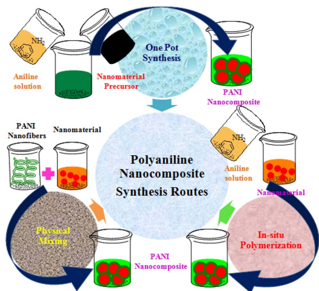
Fig. 2 Polyaniline nanocomposite synthesis routes.
