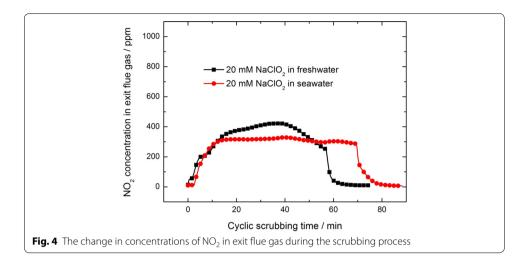
$\rm N_2$  and NO, the initial concentration of  $\rm NO_2$  in exit flue gas is zero. With the start of the scrubbing process, the concentration of  $\rm NO_2$  in exit flue gas increases gradually due to the oxidation of NO into  $\rm NO_2$  by  $\rm NaClO_2$  (Brogren et al. 1998).
