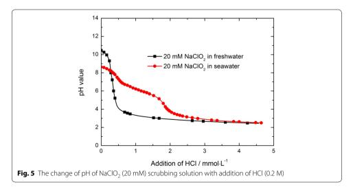
the buffering ability of seawater might be high enough to enhance the breakthrough time for NaClO<sub>2</sub> seawater during the cyclic scrubbing experiments.
