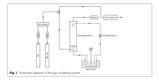
scrubbing liquid is collected under the column in a beaker, from which the absorption liquid is pumped to the top of the column using a peristaltic pump. The total amount of the cyclic scrubbing solution is 0.2 L. The rotating speed of the peristaltic pump is set at 200 rpm, resulting in that the flow rate of the scrubbing solution is about 0.35 L/min. The scrubbing solution is kept at 20 °C by immersing the beaker in a water bath.
