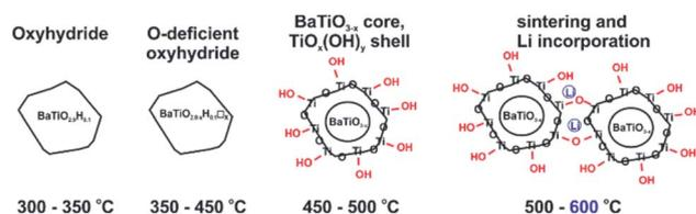
Fig. 6 Evolution of products from LiH reduction of  $\text{BaTiO}_3$  with increasing synthesis temperature.
