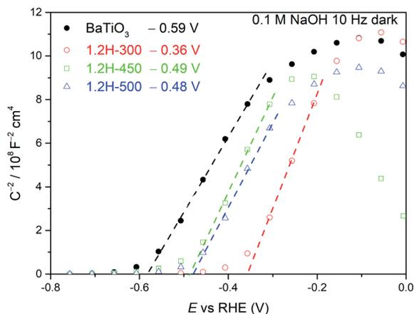
Fig. 9 Mott–Schottky plots of BaTiO<sub>3</sub>, 1.2H-300, 1.2H-450, and 1.2H-500 measured at 10 Hz under dark conditions.
