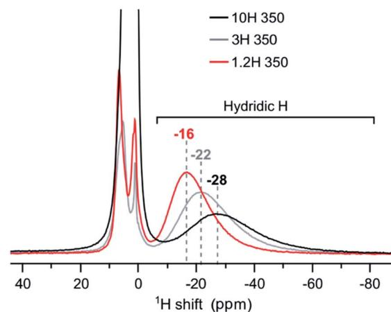
Fig. 7 <sup>1</sup>H MAS NMR spectra of products obtained from reductions using variable LiH concentrations during 48 h at 350 °C.
