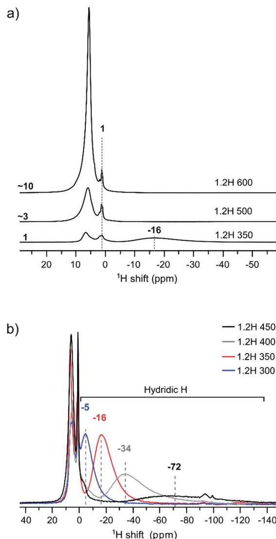
Fig. 5 (a) <sup>1</sup>H MAS NMR spectra of products obtained from 1.2 M LiH reduction during 48 h at different temperatures. The increase of protic signal (positive ppm) relative to 1.2H-350 is indicated. (b) Comparison of spectra emphasizing the negative ppm range with the hydridic H signal.
