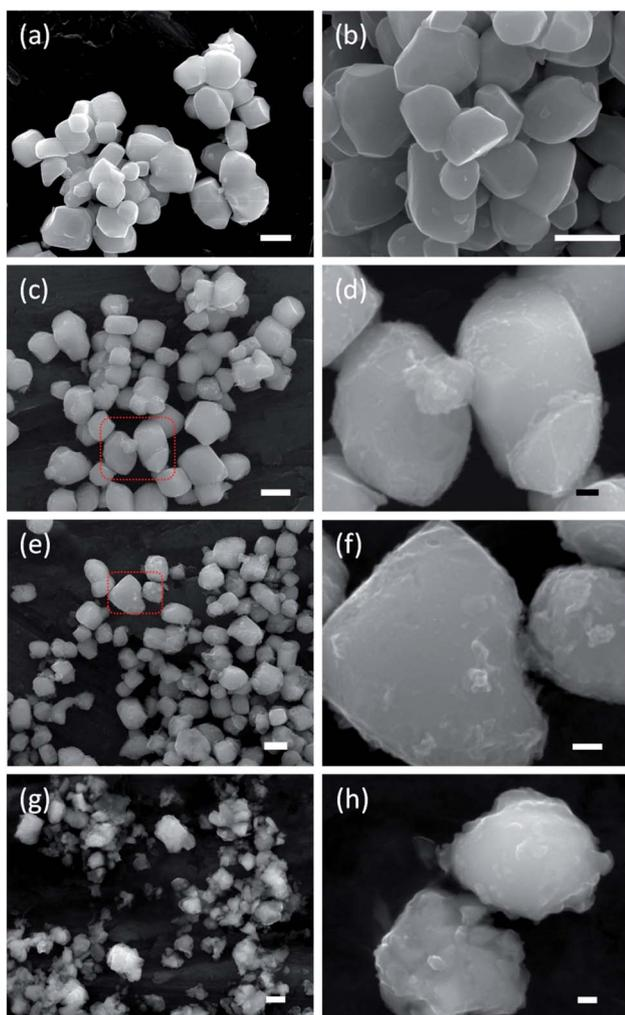
Fig. 3 SEM images of the BaTiO<sub>3</sub> starting material (a) and 1.2 M LiH reduced samples at 350 °C (b), at 450 °C (c) and (d), at 500 °C (e) and (f), and at 600 °C (g) and (h). The scale bar is 500 nm for (a)–(c), (e), (g) and 100 nm for (d), (f), (h).
