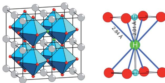
Fig. 1 The structure of BaTiO<sub>2.75</sub>H<sub>0.25</sub> represented as 2 × 2 × 2 supercell of cubic BaTiO<sub>3</sub> in which two O atoms (red circles) were randomly replaced by two H atoms (green circles). The right hand side shows the local coordination of H in BaTiO<sub>3-x</sub>H<sub>x</sub>. The Ti is in a mixed IV/III oxidation state.
