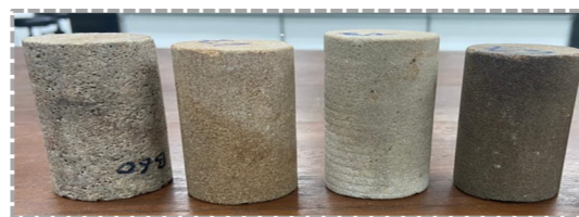
Figure 2. Sandstone core samples for oil displacement.
