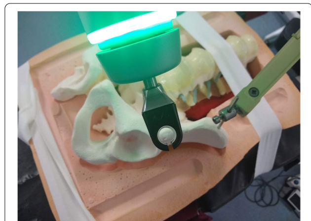
Fig. 2 View down robotic arm in preparation for LC-II screw
