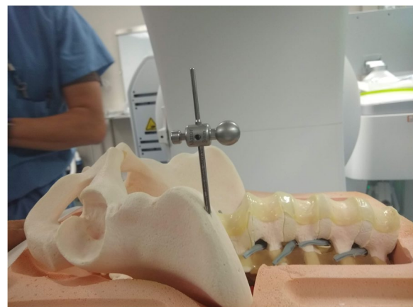
Fig. 1 Lateral view of pin placement for attachment of the robot to the model
