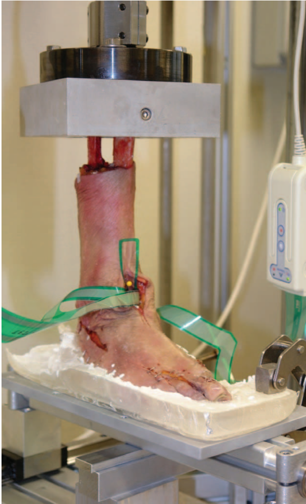
FIGURE 2. Test setup showing a specimen placed in the custom seesaw rig for ankle joint pressure and force measurements. Pressure sensors were inserted into the ankle joint in an anterior to posterior direction, being fixed with thumbtacks. Static axial compression was increased from a fixed 2-kg preload to 30 kg, according to half body weight.
