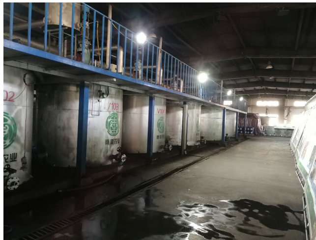
Figure 2. The reactors of the modified Fenton reaction equipment at the experimental site of Tongchuan, Shannxi, China.
