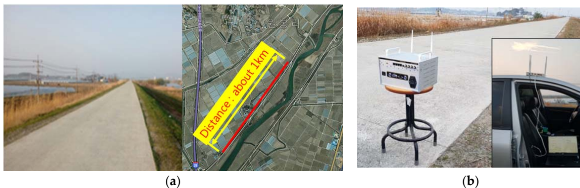
Figure 5. Test of wireless communication distance: (a) view of open field; (b) test setup in open field.
